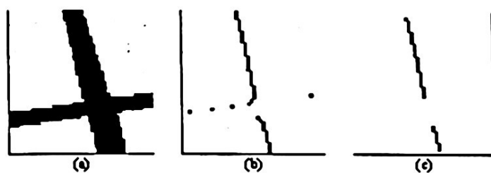
Figure 5: Vertical line extracting filter applied to the image of a crossing (a) and after edge extraction (b): result (c).
